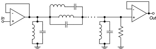
Fig. 2. Representation of the original filter based on a LC ladder, terminated with a resistor.
