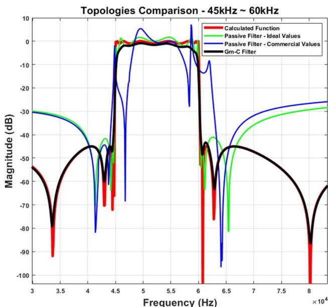
Fig. 6. Comparison of different topologies for the 45-60 kHz range.
