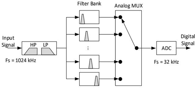
Fig. 1. The filter bank inserted in the measuring system.
